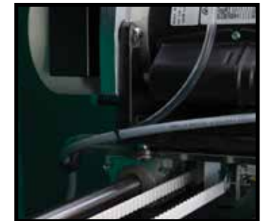
5 BELT DRIVE TRAVERSE SYSTEM ON 661 AT
