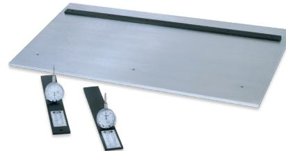
A SURFACE PLATE PROVIDES A FLAT SURFACE FOR REAR ROLLER ADJUSTMENTS, CHECKING BEDKNIFE CLEARANCES AND DETECTING FRAME ALIGNMENT PROBLEMS. MADE OF MACHINED ALUMINUM AND BUILT-IN PARALLEL BAR FOR FAST, EASY ADJUSTMENT TO THE REAR ROLLER.
